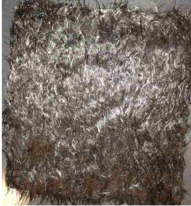
Figure 15. Recycled carbon fiber mat
