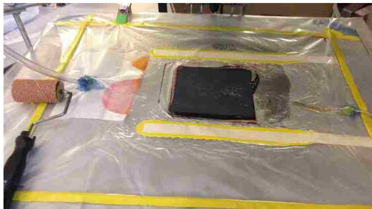
Figure 20. Vacuum Assisted Resin Transfer Molding (VARTM)
